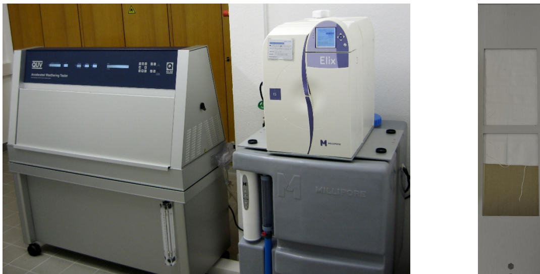
Fig. 1: Accelerated Weathering Tester QUV/SPRAY and water treatment plant type ELIX 15 (left side) and test specimen mounted on flat specimen holders (right side)
